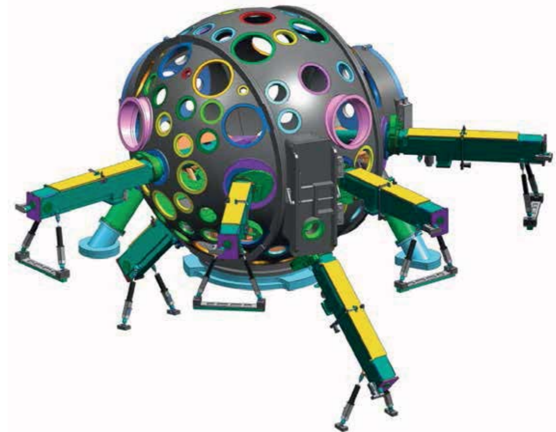
Ten Inch Manipulator Locations on the Orion target chamber.
